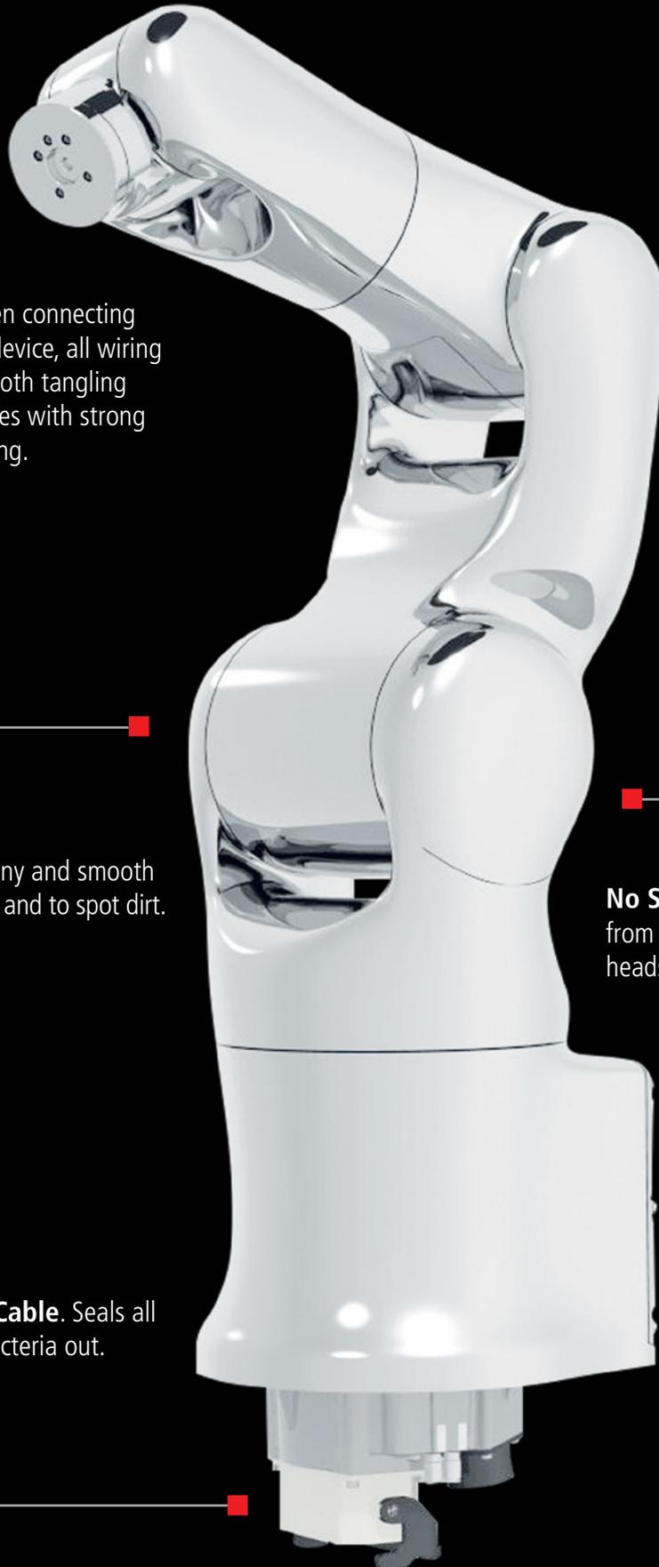
**Internal Wiring.** When connecting a flange or any other device, all wiring is internal to prevent both tangling and destroying the wires with strong chemicals while cleaning.
